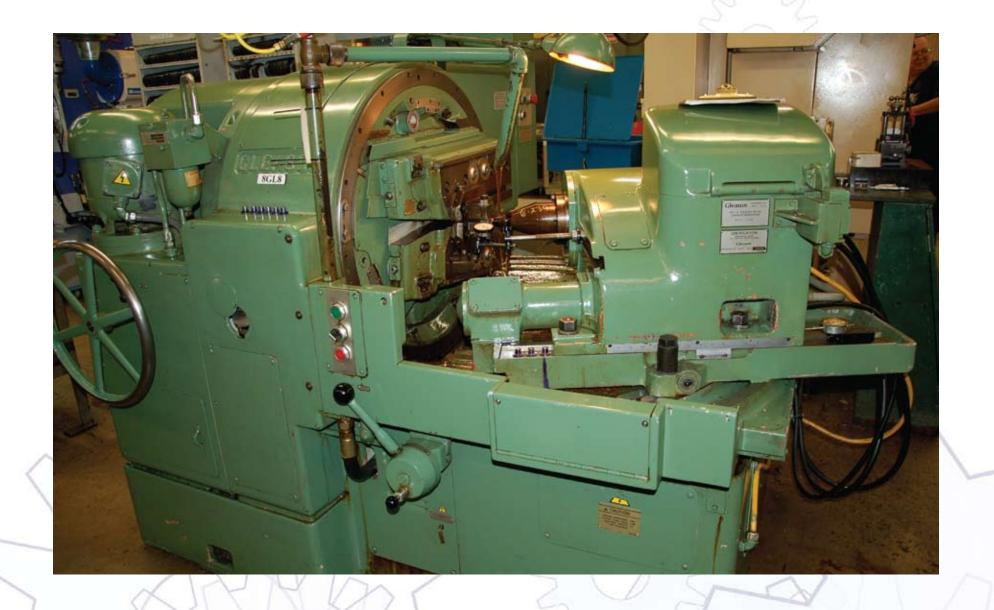
GLEASON CONIFLEX #14 Two Tool Bevel Generator
