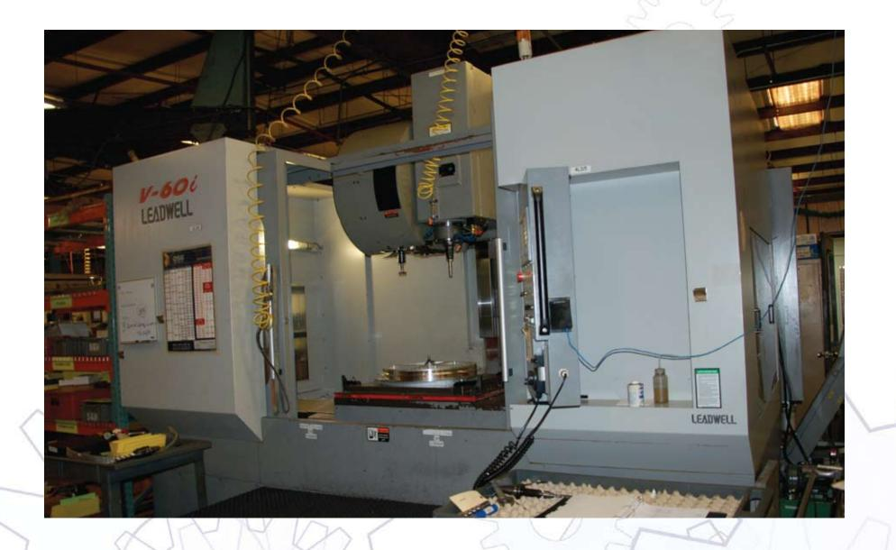
Leadwell V-60 CNC Milling Machine with 4th Axis Rotary Table
