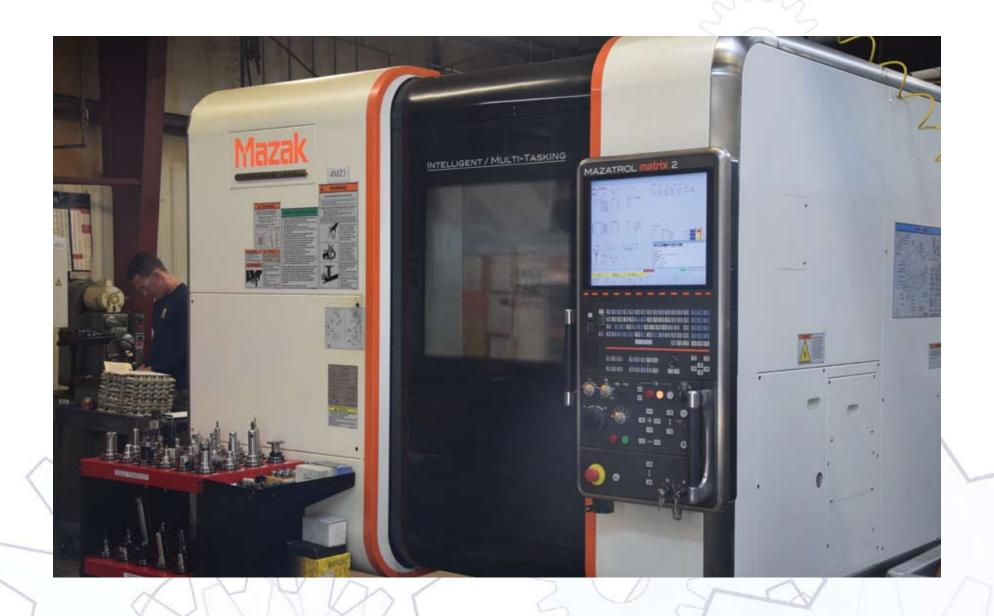
MAZAK VARIAXIS I-500 5 AXIS CNC MILLING MACHINE
