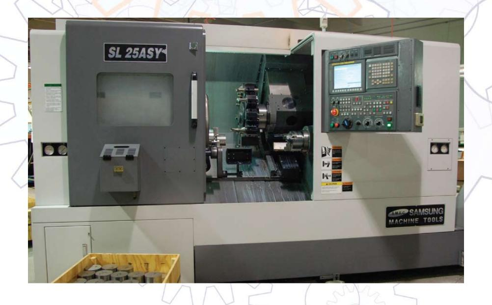
SAMSUNG SL25 ASY CNC LATHE WITH LIVE TOOLING 8" Chuck
