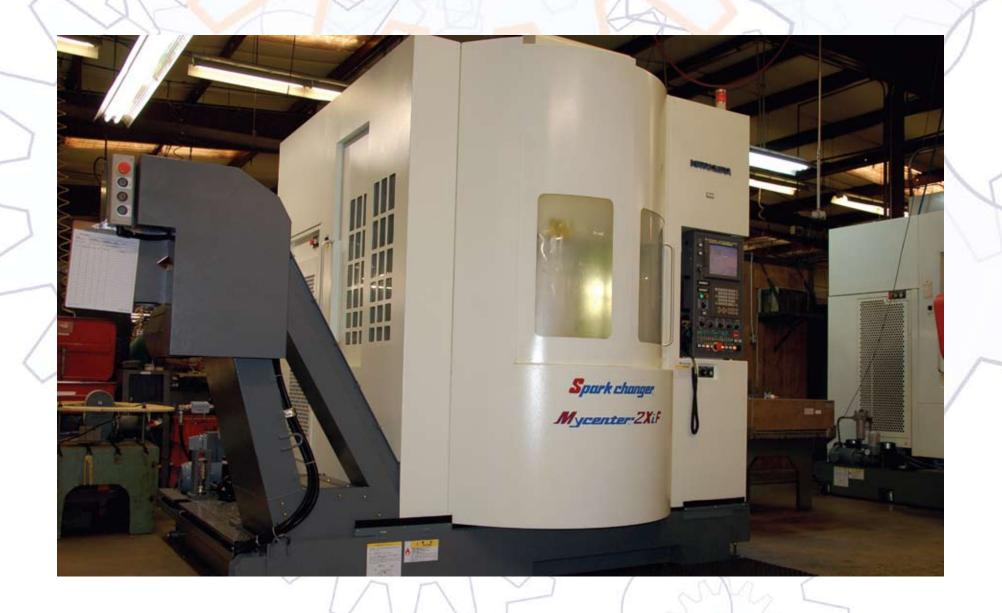
KITAMURA SPARK CHANGER MYCENTER 2X1F CNC MILLING MACHINE WITH PALLET CHANGER
